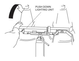
Figure 23. Pushing Down Lighting Unit
